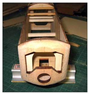
powder mixed in white glue makes excellent filler for gaps or gouges. Sand down after it dries. Use the supplied window screen material to fabricate the radiator in the opening of the cowl. Construct the under nose area of the fuselage by gluing the laminated two 1/4" balsa FB section
