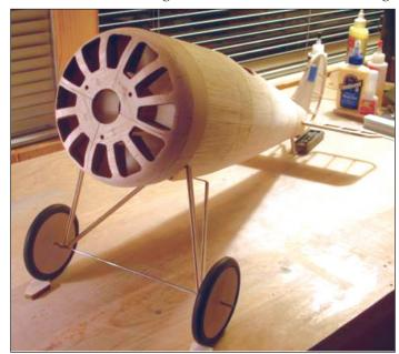
points inside the fuselage and on the bottom of the lower wing with saddle clamps. Bass wood fairings securely bound to the uprights can add significant strength. Cut the wire according to the layout on the plan. The front is in two sections to make the fabrication easier and more accurate. Bind the axle to the uprights with copper or brass wire and solder. A good alternative is to use Kevlar thread instead of
