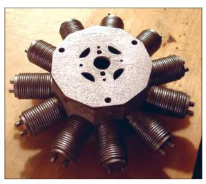
The fabrication of the engine starts with laminating the two front 1/16" ply pieces together. A 1/8" lite ply piece then gets glued to the inside face of the front ply lamination. The mounting holes for the AXI outrunner need to be drilled out to 3 mm diameter (about .120") so this was done at this time.
