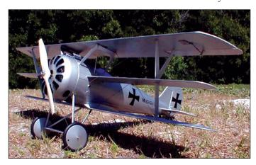
Halving the aileron down throw may reduce the yaw. This effect can be accomplished by rotating the control arm of the aileron servo forward about 20 degrees.
